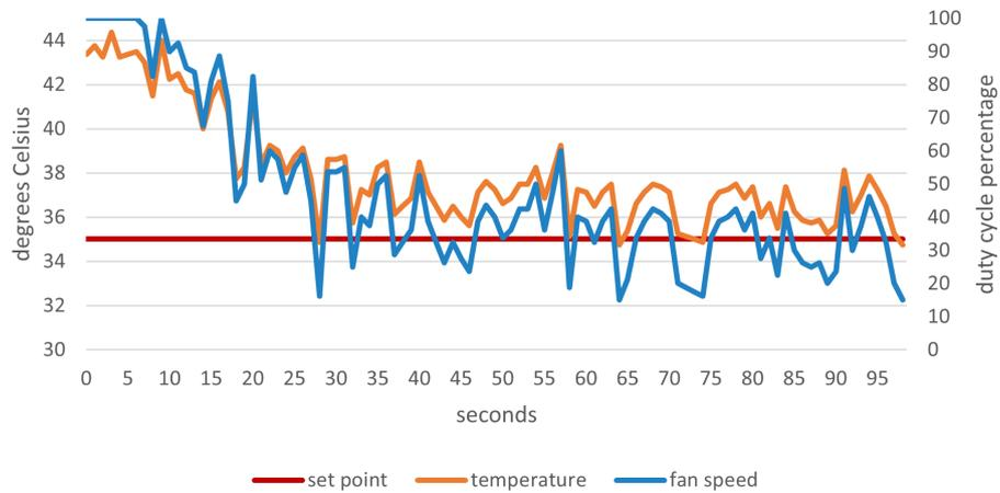
(b) Fan controller is activated after resistors
