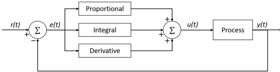
Figure 2: Block diagram of a PID controller, with feedback loop
