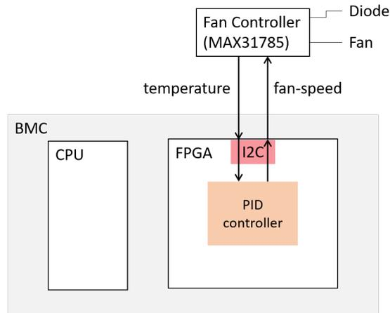
Figure 3: Diagram of the ideal integration of the PID controller into Enzian
