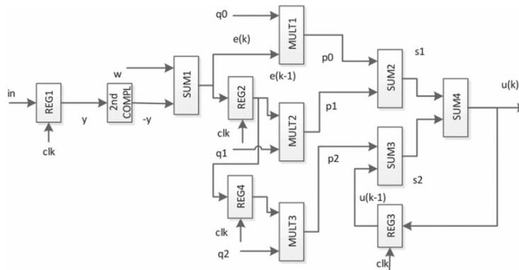
Figure 1: Parallel design of an FPGA PID controller [1]
