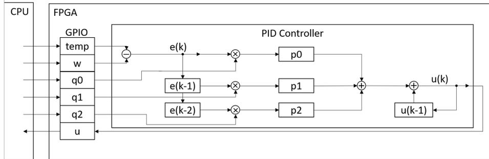
Figure 5: Simplified block diagram of the PID controller
